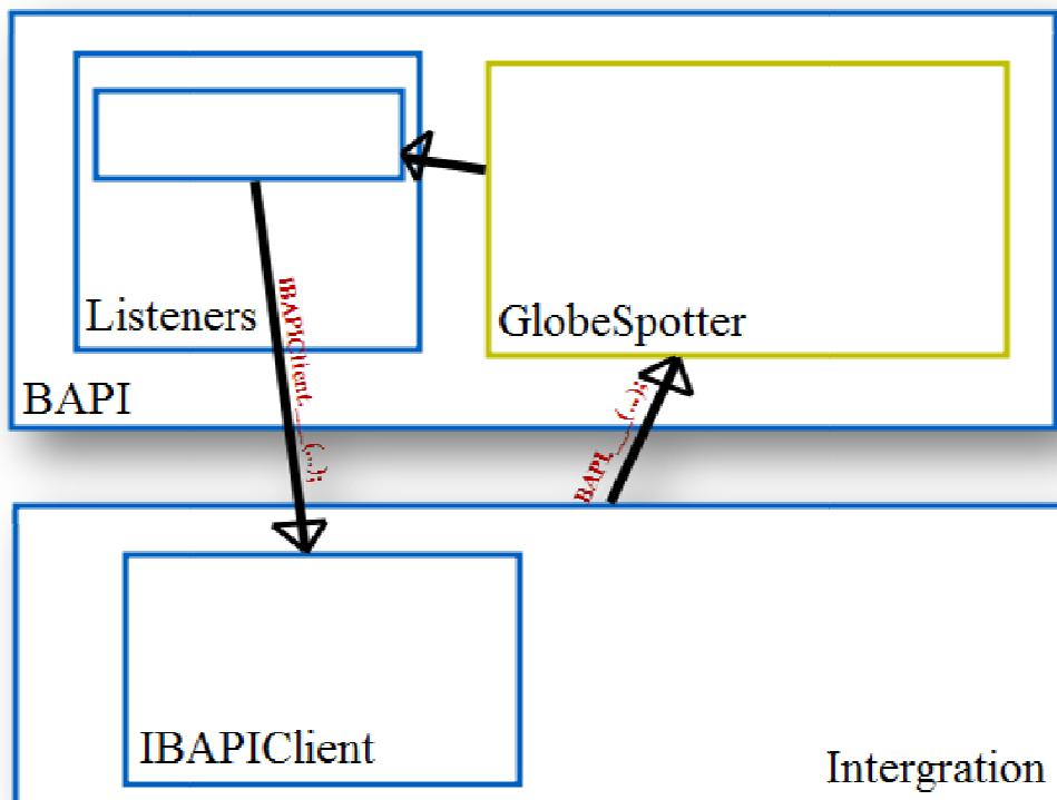
Once a *BAPI*-object is created, the integrator can add a listener (either an *IBAPIClient* or an *AbstractBAPIClient*) with the *Initialize*-method contained in the *BAPI*-class. The *Initialize*-method also initializes the process of starting-up *GlobeSpotter*, after which the integrator may expect the *OnSWFReady*-method to be called by the *BAPI*.
