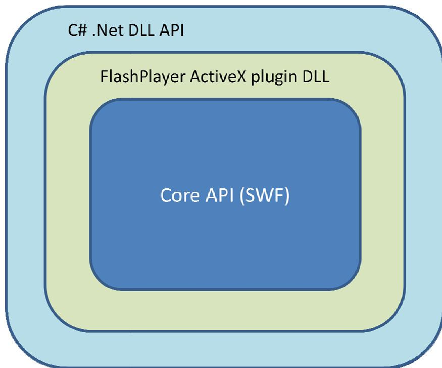
The Core API is packed in a Flash SWF component. This SWF is loaded at runtime from a remote location. The flash player is integrated in the Microsoft Windows .Net API as an ActiveX plug-in DLL. This makes it possible to use SWF components outside a web browser context. The Microsoft Windows .Net API exposes the Core API functions through a well-defined API and makes integration of this SWF component an easy task.
