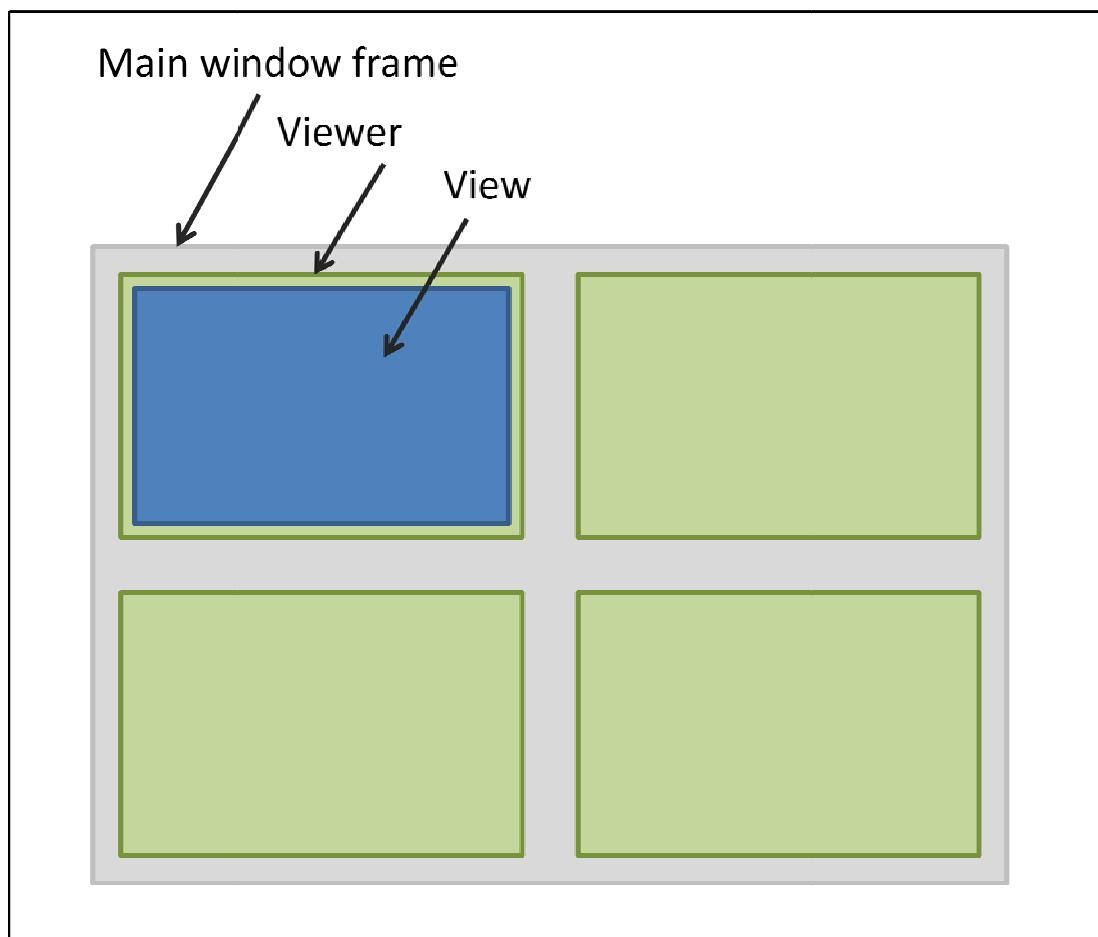
The Single Window API (BAPI) consists of a main window frame with one viewer and one view.
