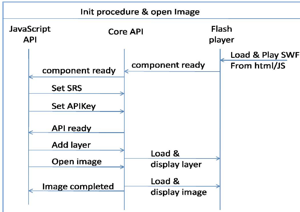
After the SWF has been loaded by the flash player, the Core API receives a Component ready event from the flash player and performs an internal initialisation procedure. When this is finished it will try to call `hst_componentReady` that should be available on the JavaScript side.
