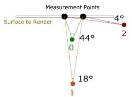
This figure demonstrates how three fictional recording locations yield varying image resolution potential, as determined by the horizontal angles between the measurement points at the surface centre.
